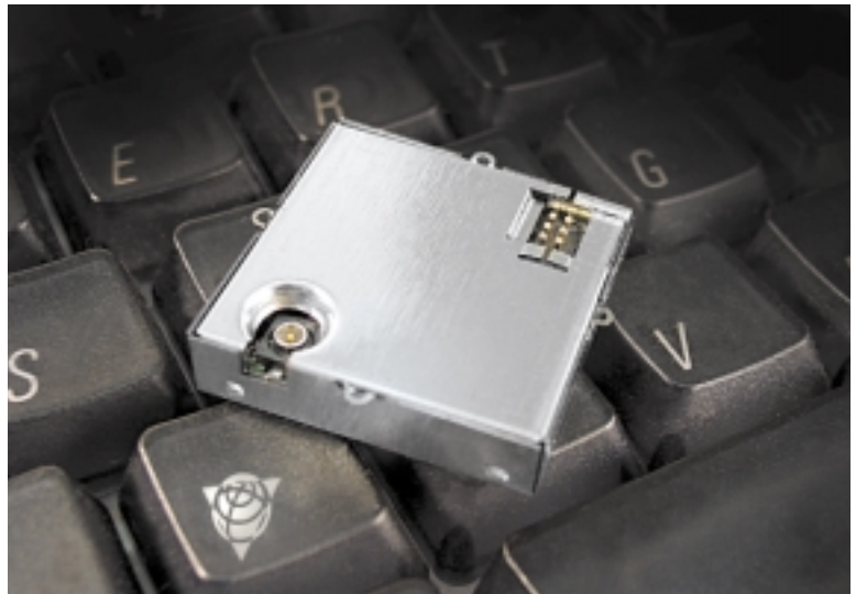
Lassen SQ GPS receiver with metal shield
